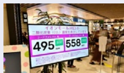
We are measuring CO 2 concentration levels in facilities. This indicates whether the ventilation rate is sufficient to maintain good indoor air quality.
